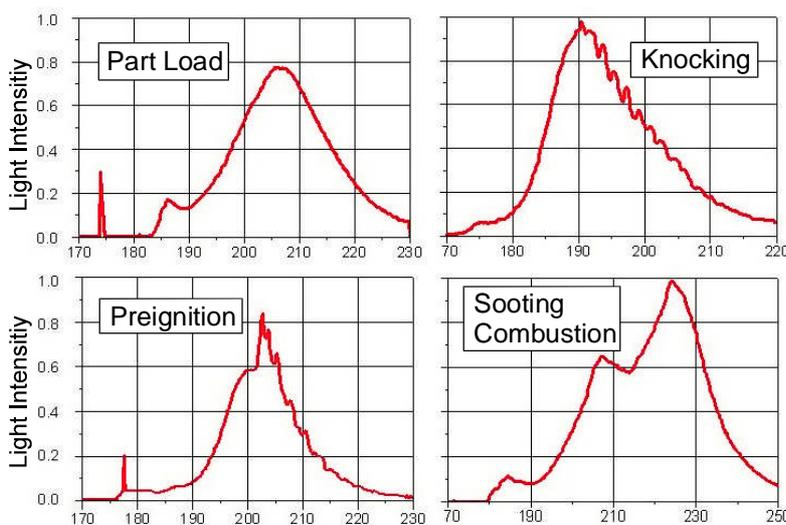
The figure beside shows different light signals detected with the FO-Spark Plug. At part load the ignition peak is very significant. After a delay the signal rises again. This is the luminosity of the flame emission mainly generated by hydro carbon radicals. The highest peak shows the radiation of all gas components in the exhaust area of the combustion chamber. The main signal is similar to the pressure signal.
