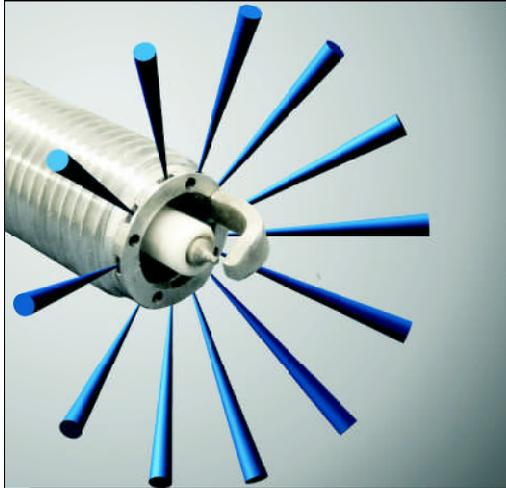
The fibre spark plug is a mass production spark plug fitted with up to 24 optical probes. The robust design of the fibre optic spark plug permits the use even at high temperature and high pressure in mass production engines. The special treatment of the spark plug does not change its thermal characteristics significantly because neither the ceramic is harmed nor the heat flow to the outer hull is handicapped.
