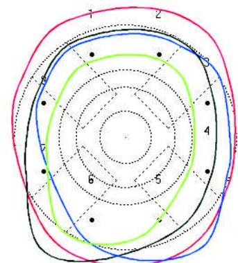
Flame kernel development of 4 subsequent combustion cycles
