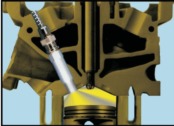
The global fibre optic measurement technique is a system to detect the combustion luminosity of a large portion of the combustion chamber. With the help of optical filters or other spectral analysis components it is possible to record the combustion process at a specified wavelength, which provides information on the gaseous components in different phases of the combustion.
